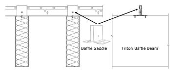
$\bf IFSS/IFSC$  internal fixing strip for screw fixing the Baffle to suspended frames such as Rondo Donn $^{\rm @}$  grid with the Baffle Saddle (IFSS) or to furring channels (IFSC).
