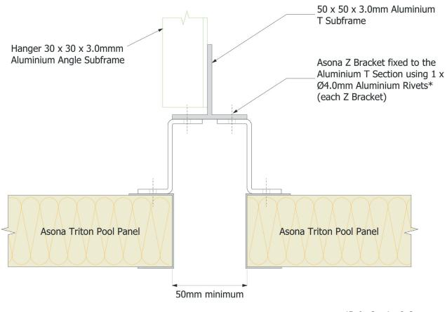
\*Refer Section 3, Components for full rivet specification
