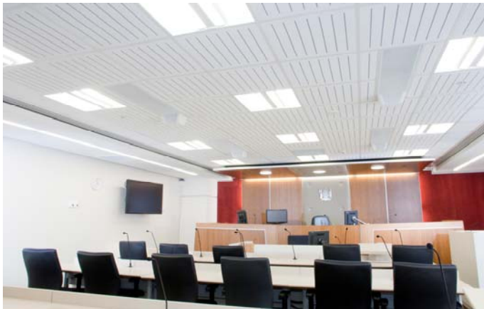
Triton 50 with Sonatex S4-500 perforated white on white facing.
