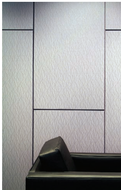
Left and top: Waiting Room, 60 mm thick Asona Sound Soft stretch fabric sound absorber wall panels with 10 mm negative for quiet comfort. Right: Danoline Tectopanel 1200 x 300 x 13mm perforated gypsum acoustic panel detail set in flush stopped plasterboard ceiling
